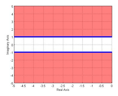
13) The (dark) shaded area in the s-plane figure below shows the possible pole location for an ideal second order system that meets which of the following constraints? a)  $PO \ge 20\%$  b)  $PO \le 20\%$
