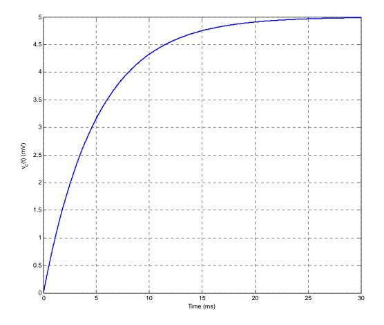
Based on this figure, the best estimate of the **time constant** for this system is a) 1 ms b) 2.5 ms c) 5 ms d) 7.5 ms e) 10 me f) 15 ms g) 30 ms
