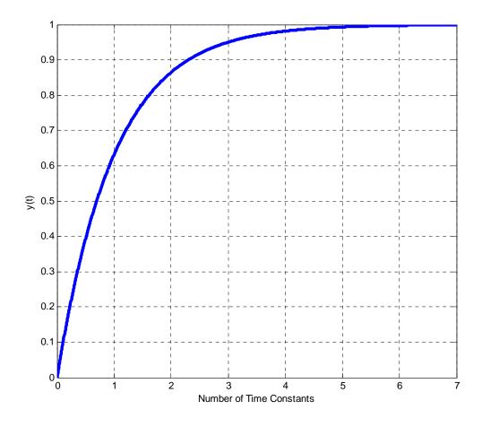
**Figure 2.6.** Graph of  $y(t) = 1 - e^{-t/\tau}$  for  $t = 0\tau$  up to  $t = 7\tau$ . y(t) is within 5% of its final value in 3 time constant, within 2% of its final value in 4 time constants, and within 1% of its final value in 5 time constants.
