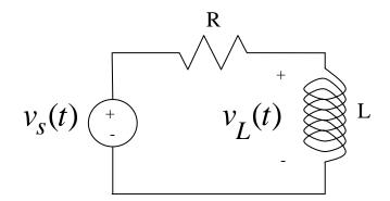
Figure 2.4. Circuit for Example 2.1.4.
