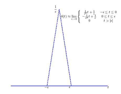
Figure 5.2. Triangular model of an impulse (delta) function.
