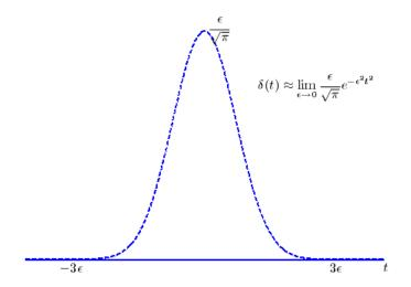
Figure 5.3. Gaussian model of an impulse (delta) function.
