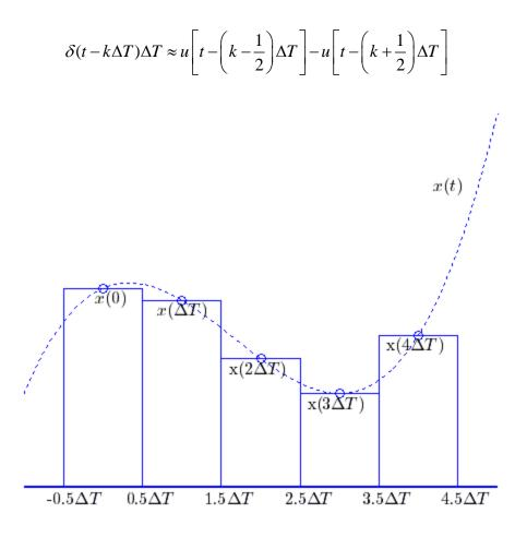
**Figure 5.6.** Approximating the continuous function x(t) as a piecewise constant function for the derivation of the convolution integral.
