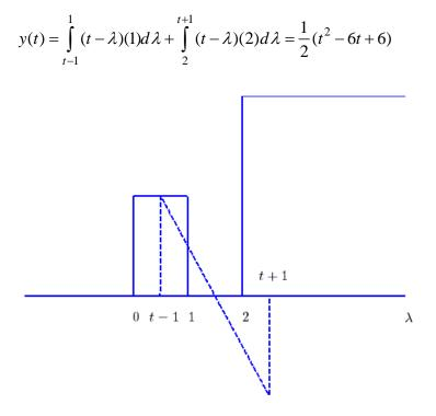
**Figure 5.16.** Third overlapping region for Example 5.5.4. This figure is valid for  $1 \le t \le 2$ .
