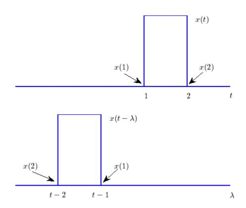
**Figure 5.7.** Input signal for Example 5.5.2. The original signal x(t) is shown in the top panel, with the two convenient "marker" points. The lower panel shows  $x(t - \lambda)$  as a function of  $\lambda$ , and shows how these marker points move as the parameter *t* is varied. Note that the function x(t) has been flipped (reversed) from its original orientation.
