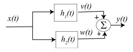
Figure 5.22. Two LTI systems connected in parallel.
