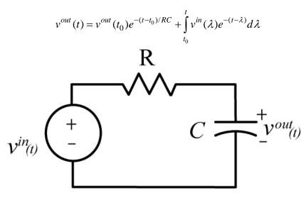
Figure 4.4. Circuit used in Example 4.1.3.
