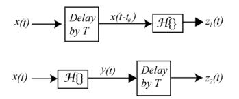
Figure 4.6. Signal flow graph of time invariance test.
