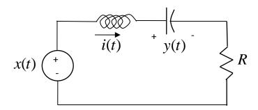
For this circuit, use your variable resistor for R, use a 0.01  $\mu$  fcapacitor, and a 33 mH inductor.
