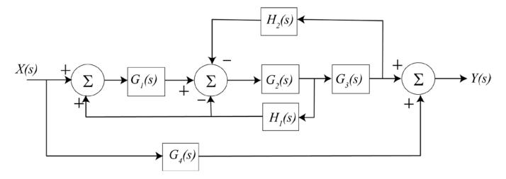
Problems 14 – 16 refer to the signal flow graph representation of the following block diagram.
