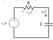
Write the output,  $V_{out}(s)$  in terms of  $V_{in}(s)$ , R, C and  $v(0^-)$ . Identify the ZSR (zero state reponse) and the ZIR (zero input response). (You can leave your answer in the s-domain)
