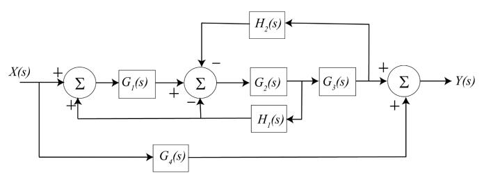
Problems 15 - 17 refer to the signal flow graph representation of the following block diagram.
