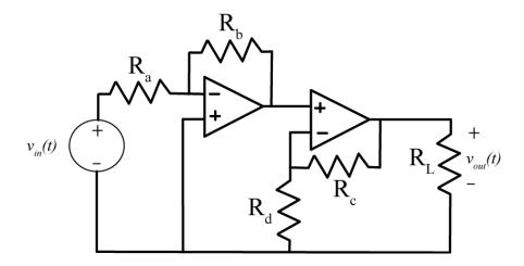
Note that the polarity of the two op-amps are different!
