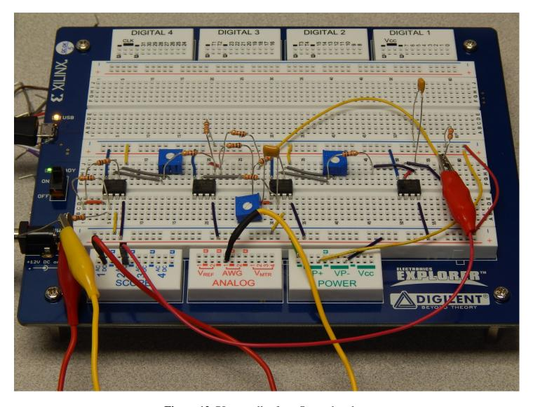
Figure 12. PI controller for a first order plant
