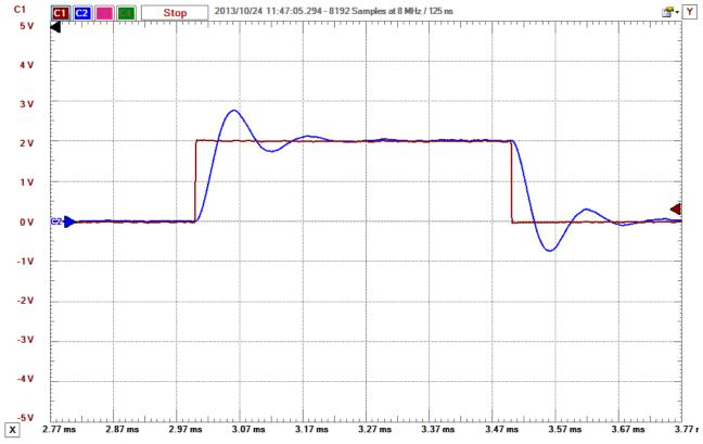
**Figure 16.** (Open loop) step response of our second order plant.
