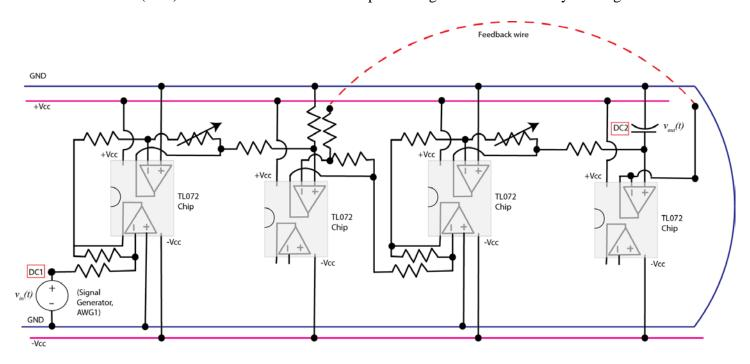
Figure 9. Closed loop system with first order plant, proportional control, and prefilter.
