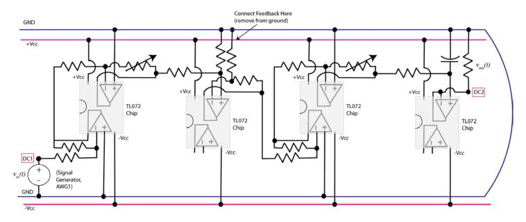
**Figure 8.** The entire system with no feedback.
