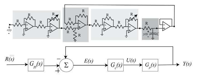
**Figure 1.** Proportional controller for the first order circuit.
