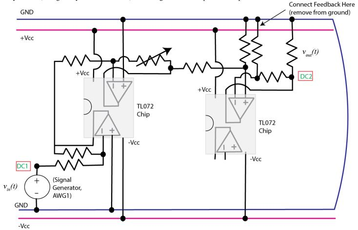
Figure 4. Prefilter and differential amplifier.
