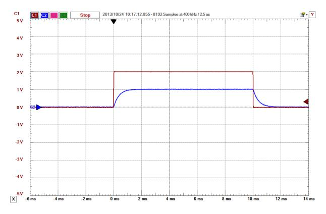
Figure 10. Closed loop response of the first order system with all gains approximately equal to one.
