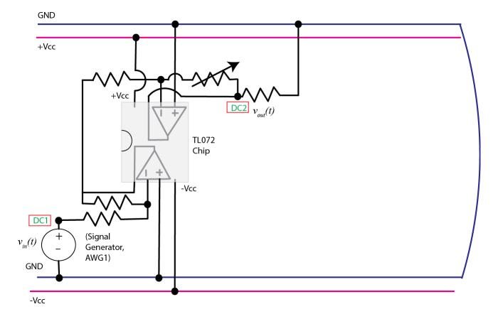
Figure 2. Prefilter (gain) circuit.
