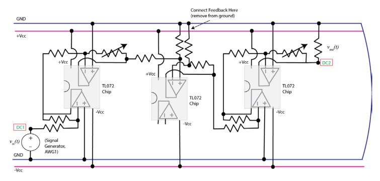
Figure 5. Prefilter, differential amplifier, and proportional controller.
