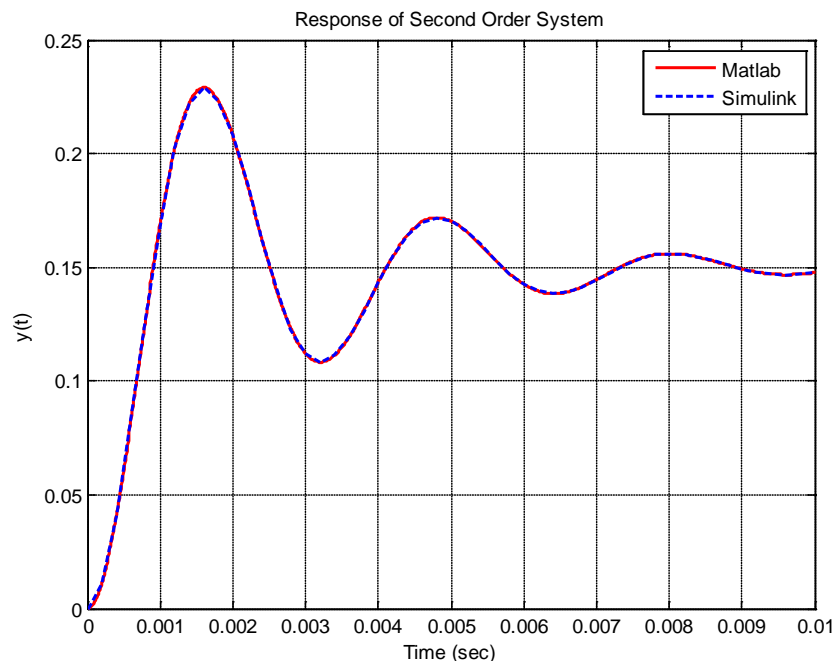
Figure 3. Response of second order system to a step of amplitude 0.1
