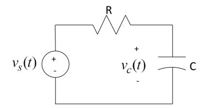
Figure 1. Circuit for Part A.
