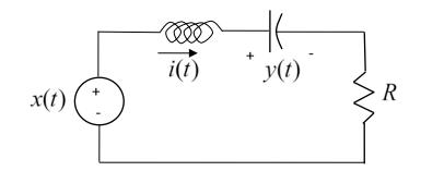
Figure 7. Second order circuit for Part C
