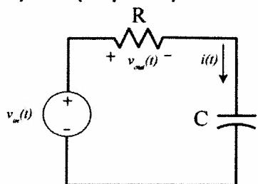
Write the output,  $V_{out}(s)$  in terms of  $V_{in}(s)$ ,  $R$ ,  $C$  and  $v(0^-)$ . Identify the ZSR (zero state response) and the ZIR (zero input response). (You can leave your answer in the s-domain)
