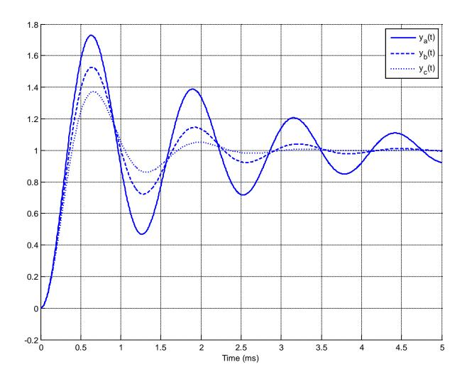
12) The following figure shows the step response of three systems. The only difference between the systems is the natural frequency,  $\omega_n$ .
