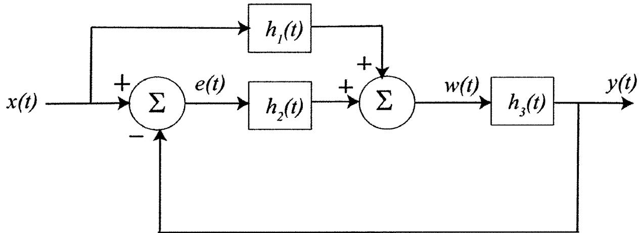
$$e(t) = x(t) - y(t) \quad w(t) = e(t) * h_2(t) + h_1(t) * x(t) \quad y(t) = w(t) * h_3(t)$$
