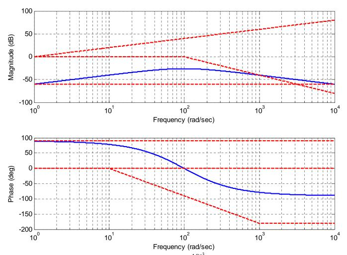
**Figure 8.17.** Bode plot for the transfer function.  $G(s) = \frac{10^{-3} s}{(0.01s+1)^2}$  The straight line approximations of
