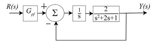
**Figure 7.15.** Block diagram for Example 7.9.3. For a unit step input, the prefilter should be one to produce zero steady state error.
