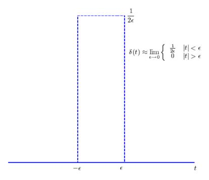
Figure 5.1. Rectangular model of an impulse (delta) function.
