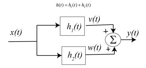
Figure 5.22. Two LTI systems connected in parallel.
