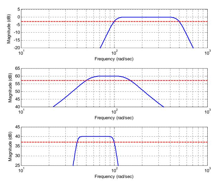
**Figure 8.22.** Three different bandpass systems with bandwidths of 400, 100, and 50 radians/sec. The -3 dB line is shown as a dashed line, and is measured from the peak amplitude.
