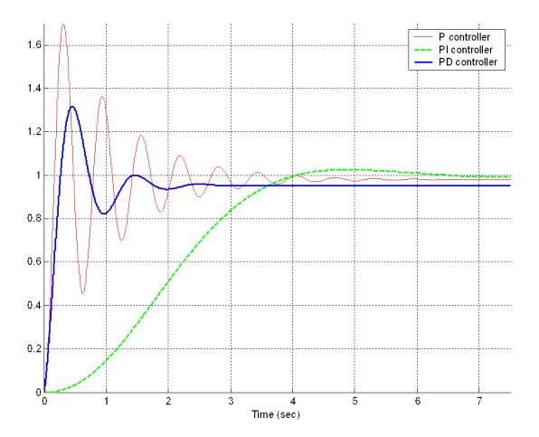
**Figure 7.18.** The response of the plant  $G_p(s) = \frac{5}{s^2 + 2s + 2}$  to the proportional (P) controller  $G_c(s) = 20$ , the proportional plus integral (PI) controller  $G_c(s) = 0.04 + \frac{0.2}{s}$ , and the proportional plus derivative controller  $G_c(s) = 8 + 0.4s$ . The input was a unit step.
