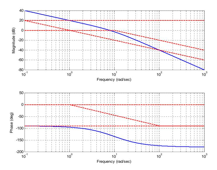
**Figure 8.15.** Bode plot for the transfer function  $G(s) = \frac{100}{s(s+10)} = \frac{10}{s(0.1s+1)}$ . The straight line
