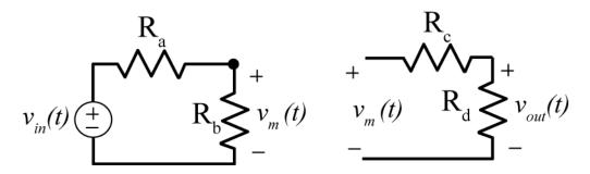
Figure 7.21. Circuit from Figure 7.20 written (incorrectly) as two subsystems.
