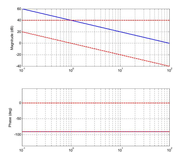
**Figure 8.12.** Bode plot of the transfer function  $G(s) = \frac{100}{s}$ . The Bode plots of the two subcomponents are shown as dashed lines, the final Bode plot is shown as a solid line. In the phase diagram, the subcomponent at -90 degrees overlaps with the final phase of -90 degrees (since the other subcomponent's phase is zero). Note that the sum of any two values (at a given frequency) on the dashed lines equals the value on the solid line at the same frequency.
