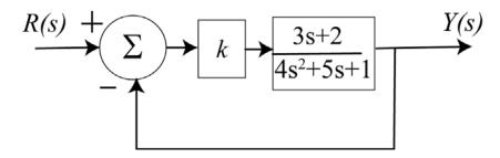
**Figure 7.16.** Block diagram for Example 7.9.4. For a unit step input, if we want the steady state error less than or equal to 0.1, we need k > 4.5.
