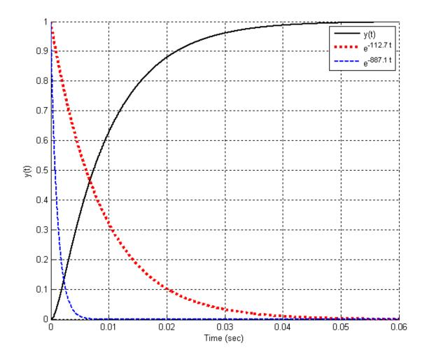
**Figure 3.12.** Response of system analyzed in Example 3.5.4 and plots of the exponentials that make up the response. For this system,  $y(t) = 1 - 1.145e^{-112.7t} + 0.145e^{-887.1t}$ . This system has components with time constants  $\tau = \frac{1}{112.7} = 0.00887 \,\text{sec}$  and  $\tau = \frac{1}{887.1} = 0.00113 \,\text{sec}$ . The response of the system is clearly dominated by the component of the response with the largest time constant.
