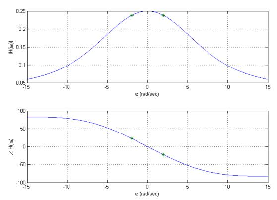
**Figure 8.8.** Plot of  $H(s) = \frac{(s+10+10j)(s+10-10j)}{(s+8+4j)(s+8-4j)(s+10)}$  as a continuous function of frequency. This is the transfer function from Example 8.3.2, and the stars (\*) denote the points we computed in that example.
