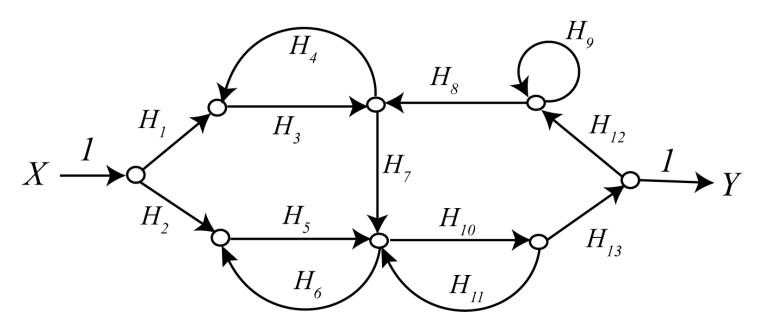
**Figure 6.16.** Example signal flow graph used in the definitions example.
