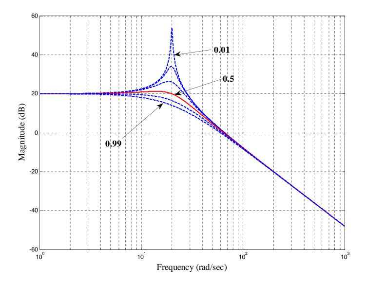
**Figure 8.18.** Magnitude of the frequency response for the transfer function  $G(s) = \frac{K\omega_n^2}{s^2 + 2\zeta\omega_n s + \omega_n^2}$  for  $K = 10, \omega_n = 20$ , and  $\zeta = 0.01, 0.1, 0.250.5, 0.75, 0.99$
