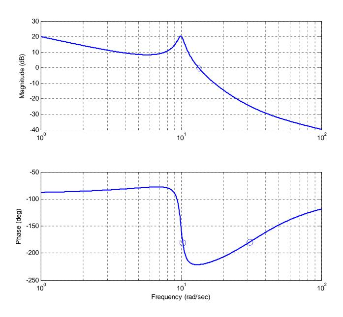
**Figure 8.28**. Bode plot for Example 8.7.3. The gain crossover frequency is shown as a diamond, and the two phase crossoever frequency is shown as the open circles.
