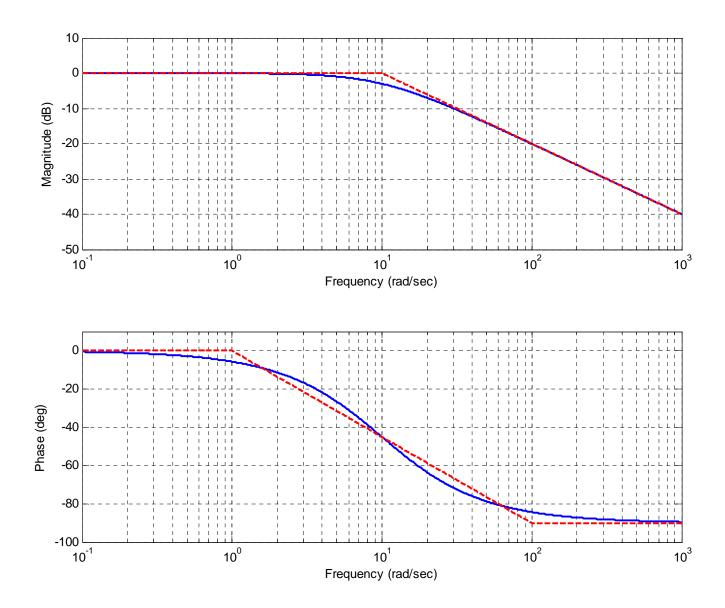
**Figure 8.13.** Bode plot for the transfer function  $G(s) = \frac{1}{0.1s+1}$ . Note the 3 dB discrepancy at the corner frequency in the magnitude plot. The Bode plot of the straight line approximation is shown as dashed lines while the exact Bode plot is shown as a solid line.
