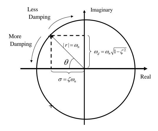
**Figure 7.5.** Relationship between damping ratio ( $\zeta$ ), natural frequency ( $\omega_n$ ), and damped frequency ( $\omega_d$ ) in the complex plane for an under damped system ( $0 < \zeta < 1$ ). The poles of the system are located at  $s = -\sigma \pm j\omega_d$ .
