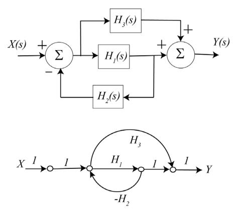
Figure 6.17. Block diagram and signal flow graph for Example 6.7.4.
