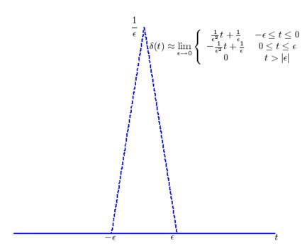
Figure 5.2. Triangular model of an impulse (delta) function.
