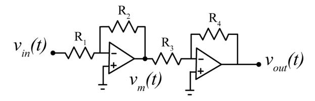
Figure 7.14. Proportional gain circuit for Example 7.7.1.
