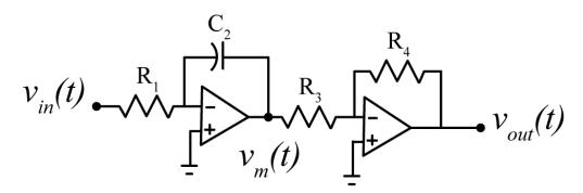
**Figure 7.15.** Integral and gain op amp circuit for Example 7.7.2.
