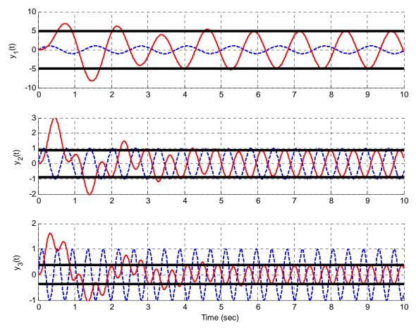
**Figure 8.2.** Response of the second system to sinusoids of 5, 10, and 15 radians/sec. The estimated settling time of the system is 6.7 seconds. The input signal is the dashed line and the output signal is the solid line. The thick solid line bounds the steady state amplitude.
