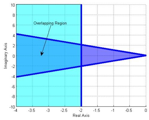
**Figure 7.10.** The pole locations corresponding to a maximum percent overshoot of 5% and a settling time of 2 seconds are shown in the shaded regions. The overlapping region shows the location in the *s*-plane where both conditions are met.
