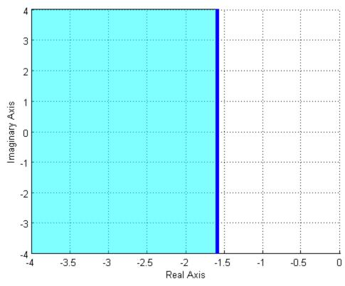
**Figure 7.6.** The pole locations corresponding to a settling time less that 2.5 seconds are shown in the shaded region, to the left of -1.6 on the real axis. Note that the settling time constraint only affects the real part of the pole, not the imaginary part of the poles.
