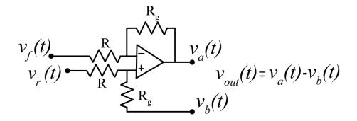
**Figure 7.16.** Differential amplifier circuit used in Example 7.7.3.
