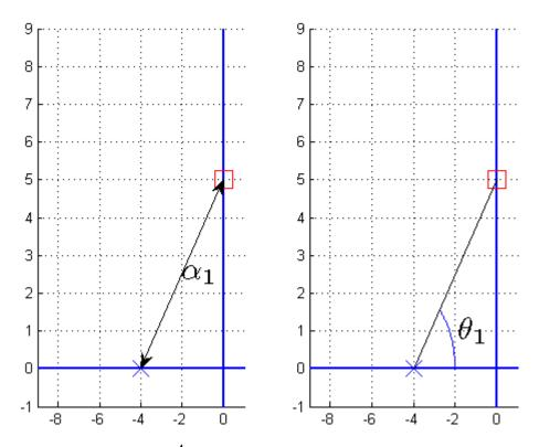
**Figure 8.4.** Pole-zero plot of  $H(s) = \frac{4}{s+4}$  evaluated at 5 radians/second. The distance between the pole and the point j5 is used in the magnitude computation, while the angle between the pole and the point j5 is used in the phase computation.
