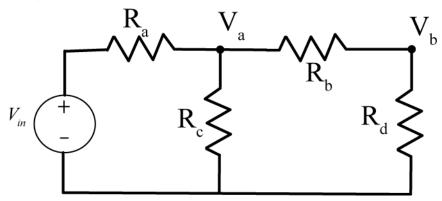
**b)** Create m-files to set up and solve matrix equations for the node values for the following circuit. Use **both** methods from the Appendix to set up the system of equations.
