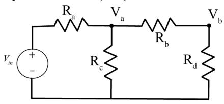
We can write node equations at these two nodes as
