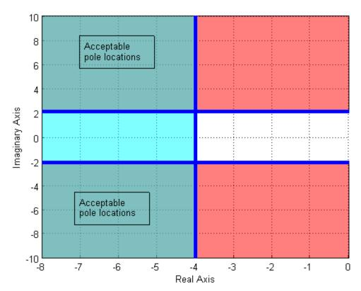
**Figure 7.12.** The pole locations corresponding to a maximum time to peak of 1.5 seconds and a settling time less than 1 seconds. The settling time constraint means the real part of the poles must be let than -4, and the peak time constraint means the absolute value of the imaginary part of the pole must be greater than 2.09. The pole locations that meet both of these constraints is the overlapping regions, labeled as "Acceptable pole locations".
