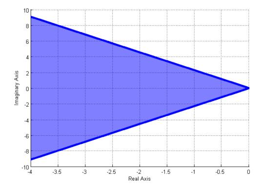
**Figure 7.8.** The pole locations corresponding to a maximum percent overshoot of 25% are shown in the shaded region, within the wedge.. Note that the percent overshoot affects both the real and imaginary parts of the poles.
