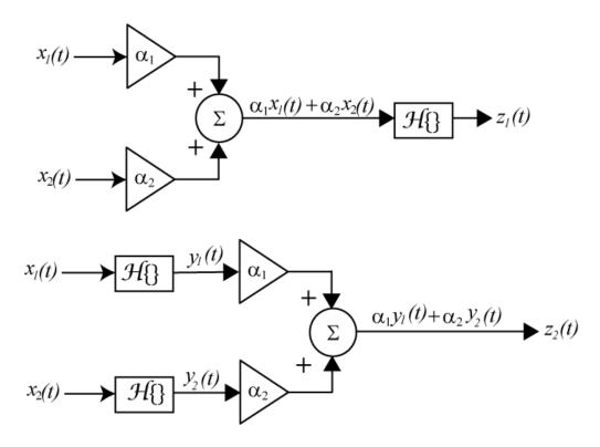
**Figure 4.5.** Signal flow graph of linearity test.
