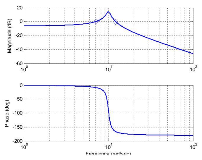
**Figure 8.27.** Bode plot for Example 8.7.2. The gain crossover frequencies are shown as diamonds. There is no phase crossover frequency. The phase margin for this system is approximately 14 degrees, and the gain margin is infinte.
