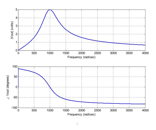
**Figure 1.** Frequency response of the Sallen-Key filter from problem 11.
