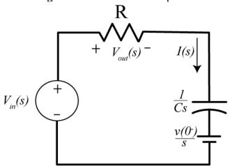
**Figure 6.5.** Circuit from Example 6.3.1 in the Laplace domain.
