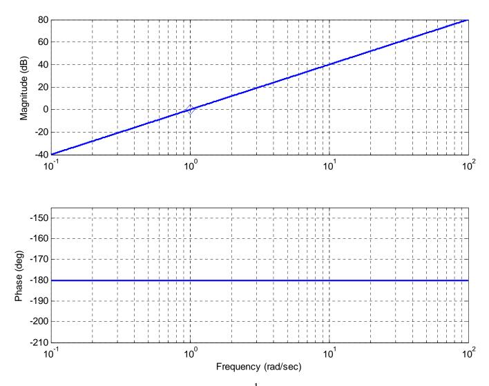
**Figure 8.11.** Bode plot of the transfer function  $G(s) = \frac{1}{s}$ . Note that a diamond delineates the point (1 rad/sec, 0 dB).
