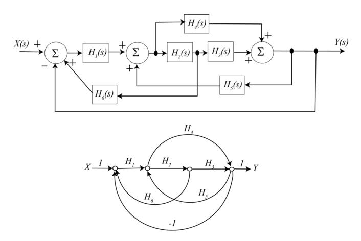
Figure 6.19. Block diagram and signal flow graph for Example 6.7.6.
