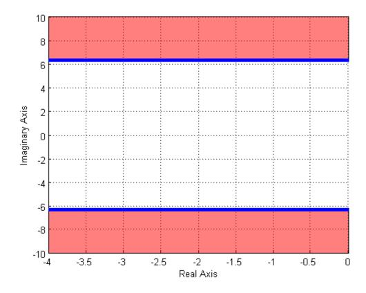
**Figure 7.11.** The pole locations corresponding to a maximum time to peak of 0.5 seconds. This corresponds to the imaginary part of the poles being larger than 6.28. Note that this constraint affects only the imaginary parts of the pole.
