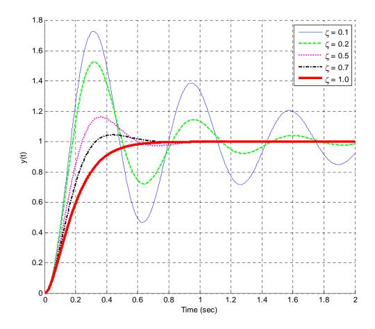
**Figure 3.6.** The response (output) of a system initially at rest. For this system KA = 1 and  $\omega_n = 10$  rad/sec. There are four responses for under damped systems ( $0 < \zeta < 1.0$ ) and one response for a critically damped system ( $\zeta = 1.0$ ). The only thing changing in the responses is the damping ratio.
