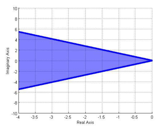
**Figure 7.9.** The pole locations corresponding to a maximum percent overshoot of 10% are shown in the shaded region, within the wedge. Note that the percent overshoot affects both the real and imaginary parts of the poles. Note also that the angle of this wedge is narrower than that in Figure 7.8 since the allowed percent overshoot in that case is smaller (10% compared to 25% in Figure 7.8).
