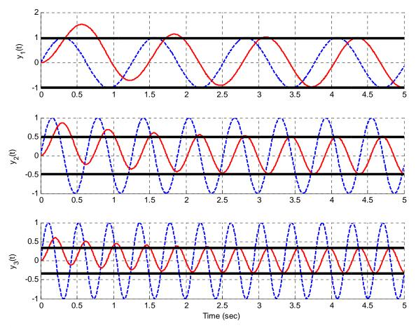
**Figure 8.1.** Response of the first system to sinusoids of 5, 10, and 15 radians/sec. The estimated settling time of the system is 4 seconds. The input signal is the dashed line and the output signal is the solid line. The thick solid line bounds the steady state amplitude.
