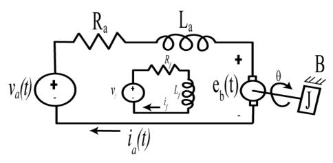
Figure 7.18. Model of an armature controlled DC motor.
