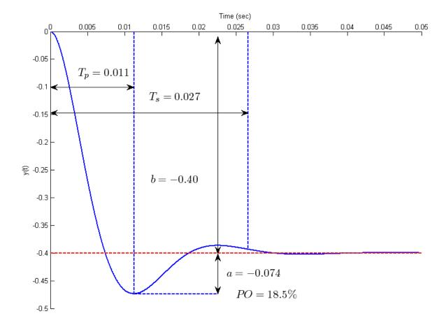
**Figure 3.9.** Response of the circuit used in Example 3.5.2 with parameter values  $C_a=10~\mu F$ ,  $C_b=1~\mu F$ ,  $R=1~k\Omega$ ,  $R_a=3~k\Omega$ ,  $R_b=2~k\Omega$ . The input is a 1 volt step. Note that although the input to the circuit is a positive voltage, the output is negative because the static gain is negative.
