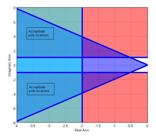
**Figure 7.13.** The acceptable pole locations for an ideal second order system that corresponds to a time to peak of less than or equal to 3 seconds, a settling time of less than 2 seconds, and a percent overshoot of less than 20%. The pole locations that meet all of these constraints is the overlapping regions, labeled as "Acceptable pole locations".
