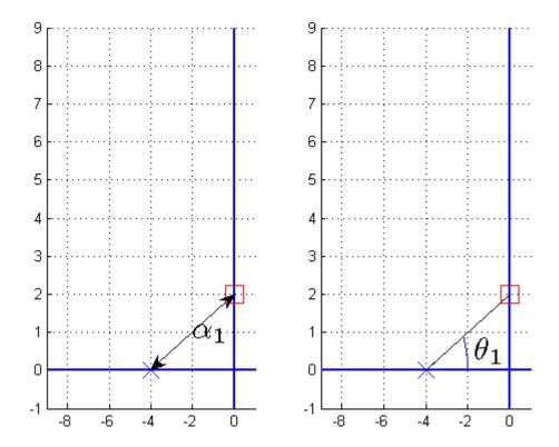
**Figure 8.3.** Pole-zero plot of  $H(s) = \frac{4}{s+4}$  evaluated at 2 radians/second. The distance between the pole and the point j2 is used in the magnitude computation, while the angle between the pole and the point j2 is used in the phase computation.
