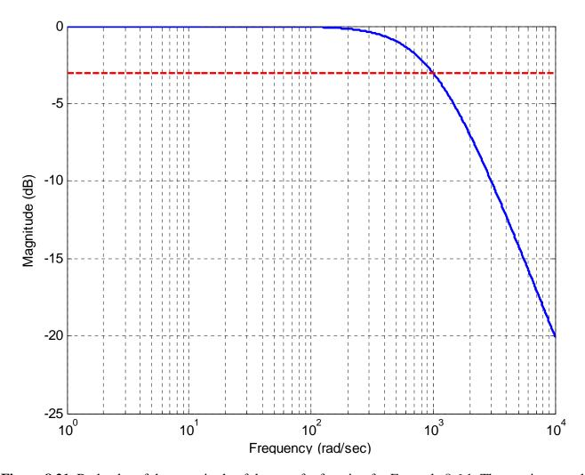
**Figure 8.21.** Bode plot of the magnitude of the transfer function for Example 8.6.1. The maximum value of the transfer function is 1 (0 dB), so the bandwidth will be determined by the point where the magnitude falls to -3dB. This occurs at 1000 rad/sec.
