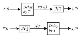
Figure 4.6. Signal flow graph of time invariance test.
