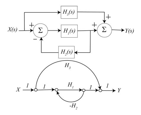
Figure 6.18. Block diagram and signal flow graph for Example 6.7.5.
