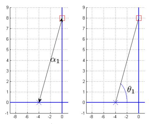
**Figure 8.5.** Pole-zero plot of  $H(s) = \frac{4}{s+4}$  evaluated at 8 radians/second. The distance between the pole and the point j8 is used in the magnitude computation, while the angle between the pole and the point j8 is used in the phase computation.
