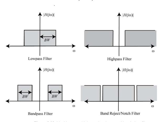
**Figure 8.23.** Ideal lowpass, highpass, bandpass, and bandreject filters.
