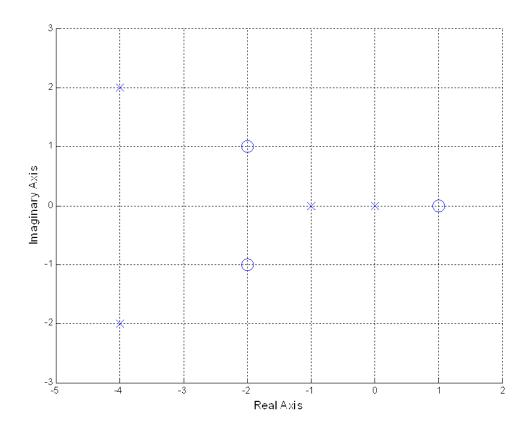
**Figure 6.10.** Pole-zero plot for transfer function of Example 6.5.1.
