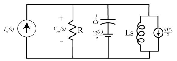
**Figure 6.9.** Circuit from Example 6.3.3 in the Laplace domain.
