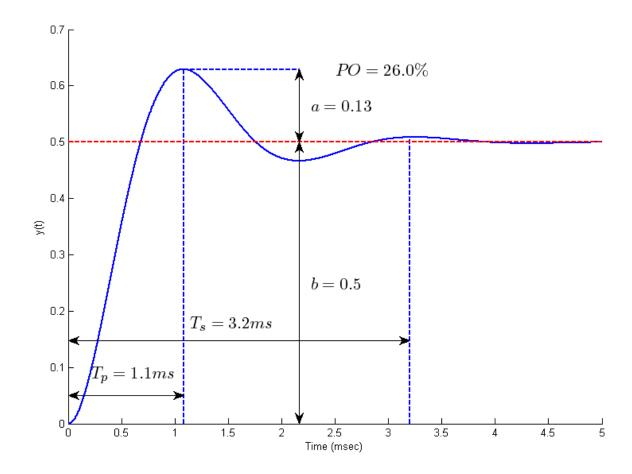
**Figure 3.8.** Response of the circuit used in Example 3.5.1 with parameter values L = 10 mH ,  $C = 10 \mu$ F ,  $R = 40 \Omega$  . Assume the input is 0.5 amp step.
