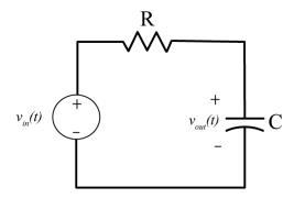
Figure 8.20. RC circuit for Example 8.6.1.
