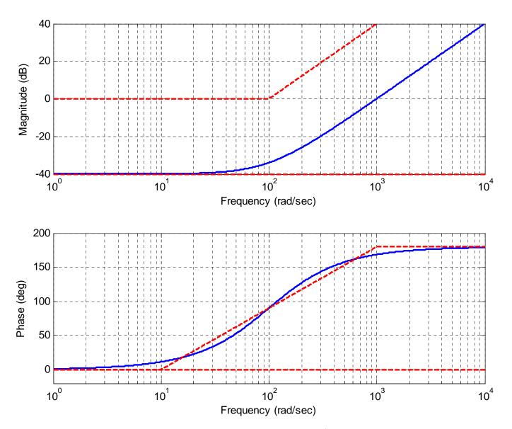
**Figure 8.14.** Bode plot for the transfer function  $G(s) = \frac{1}{100} \left( \frac{1}{100} s + 1 \right)^2$ . Note the 6 dB discrepancy at
