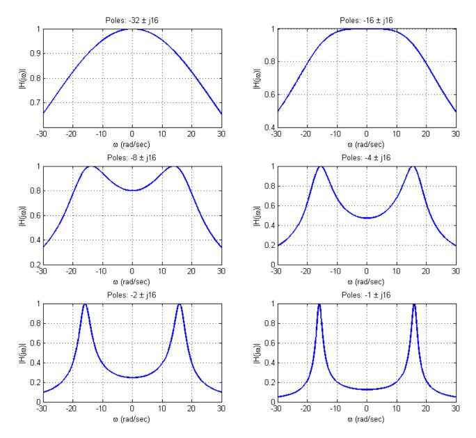
**Figure 8.9.** This figure shows the magnitude of the frequency response of various systems that have two complex conjugate poles. All of these systems have poles of the form  $\sigma \pm 16$  where the real part of the pole varies from -32 to -1. The magnitudes for these systems have been scaled to have a maximum value of one.
