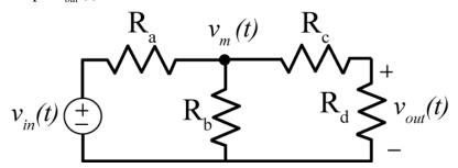
**Figure 7.20.** Circuit used to demonstrate loading.
