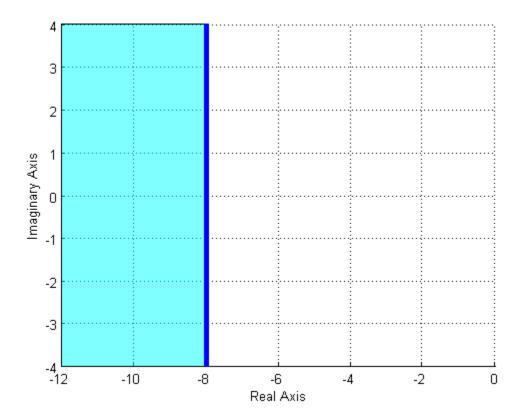
**Figure 7.7.** The pole locations corresponding to a settling time less that 0.5 seconds are shown in the shaded region, to the left of -8 on the real axis. Note that the settling time constraint only affects the real part of the pole, not the imaginary part of the poles.
