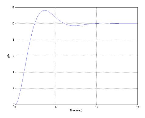
**Figure 7.4.** Response of system for Example 7.5.2 to a step of amplitude 5. The static gain of this system is 2 and the final value of the output is then 10, as the figure shows.
