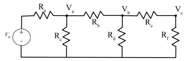
c) Create m-files to set up and solve matrix equations for the node values for the following circuit. Use *both* methods from the Appendix to set up the system of equations.
