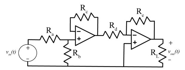
5) For the following circuit, show that  $v_{out}(t) = \left(-\frac{R_b}{R_a} \frac{R_c + R_d}{R_d}\right) v_{in}(t)$
