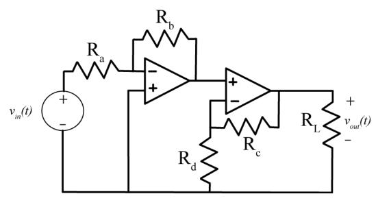
Note that the polarity of the two op-amps are different!
