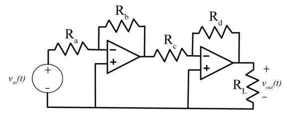
**4)** For the following circuit, show that  $v_{out}(t) = \left(-\frac{R_e}{R_d} \frac{R_b}{R_a + R_b}\right) v_{in}(t)$
