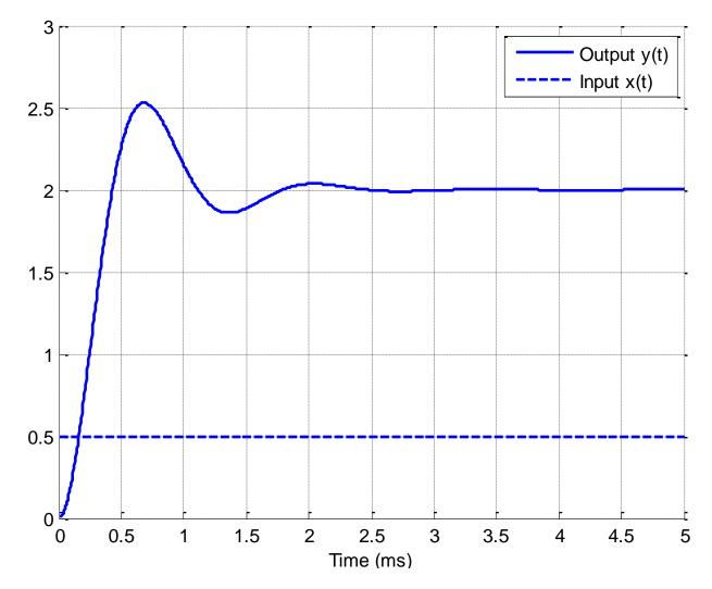
Problems 8-11 refer the following graph showing the response of a second order system to a step input.
