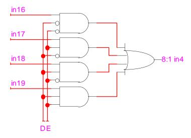
Making one sub-circuit for each of the eight inputs leads to the final circuit:
