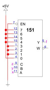
2. Implement a 32:1 multiplexer with active-low enable using only ONE 74LS151 multiplexer and any glue logic (AND, OR, NOT, etc.) that you desire. Build your circuit using simulation software. NOTE: you should not try to test this circuit with all 2<sup>32</sup> inputs!!!
