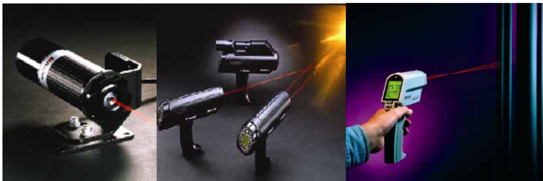
Fig. 16: Devices with laser sighting allow a precise spot measurement even of small objects.
