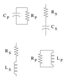
It's important to recognise that the values of the components in the two types of model are not equal, though they are related. For the capacitor,
