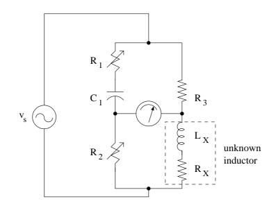
In Hay's bridge,  $R_1$  is in series with  $C_1$ . Hay's bridge is less convenient for measuring inductances, as its balance equations
