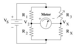
This bridge consists of two resistor branches: on the left are two precision resistors  $R_1$  and  $R_2$ . On the right are a precisely calibrated variable resistor  $R_3$  and an unknown (or imprecisely known) resistor  $R_X$ . If the current flowing between the mid-points of the branches happens to be zero, then the branches will function as accurate voltage dividers, in which case the voltage across  $R_2$  will be
