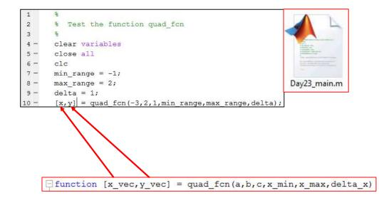
This passing of the variables back and forth can be seen clearly when you run the DEBUGGER with a function like this. You can try this on your own as well.
