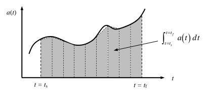
The approximate area under the acceleration curve can be given by
