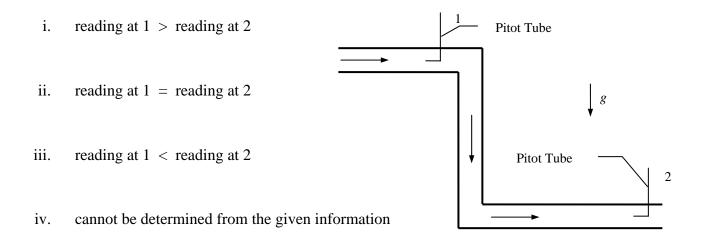
d) Low-speed air flows through a diverging section of a diffuser. Two Pitot tubes are loated as shown and attached to pressure gages. In the ABSENCE of fluid friction, which one of the following statements correctly compares the pressure measurement on the two Pitot tubes?
