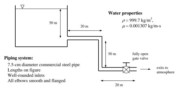
**Part (b) (65 points)** --- A turbine is added to the exit of the piping system described in Part (a) as shown in the figure below. The water velocity in the pipe is 5 m/s when the turbine is operating and *friction effects cannot be neglected* in the piping system.
