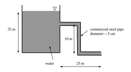
(b) With fluid friction taken into account, what is the value of h so that the same flow speed as that in Part (a) is to be sustained in the following system? Assume all 90° bends are smooth and threaded.
