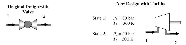
The adiabatic turbine is designed to operate with negligible changes in kinetic energy and gravitational potential energy at steady-state conditions.
