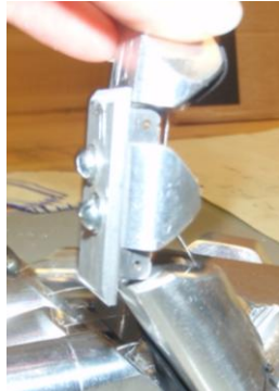
Figure 6: Metal plate to prevent backwards motion
