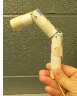
Figure 2: First prototype, string run through center to bend finger
